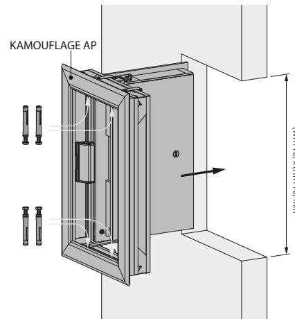
2. Make an opening with dimensions  $(W+10) \times (H+10)$  mm.
