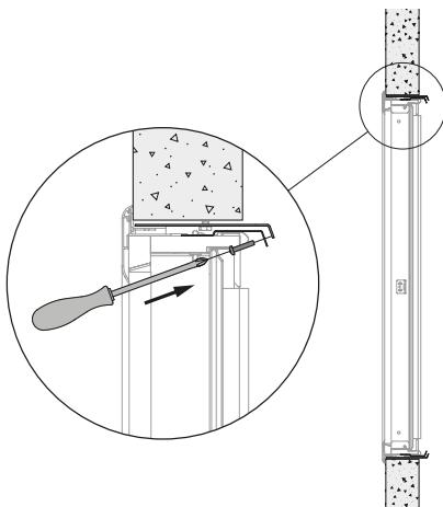
5. Open the shutter and position it in the mounting frame. Fasten the shutter onto the mounting frame with the 4 screws supplied, as shown in the drawing. Tightening the screws pulls the shutter towards the wall until its final position. You can also slightly correct the angle of the shutter with respect to the mounting frame. Connect the mechanism according to the wiring diagram.
