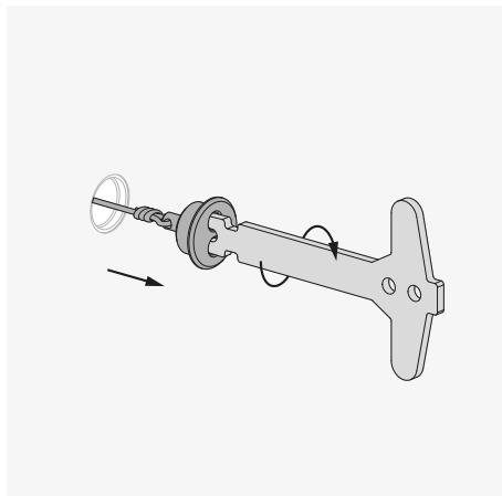
1. Unscrew the finishing cap from the opening in the door. Use the key to do this.
