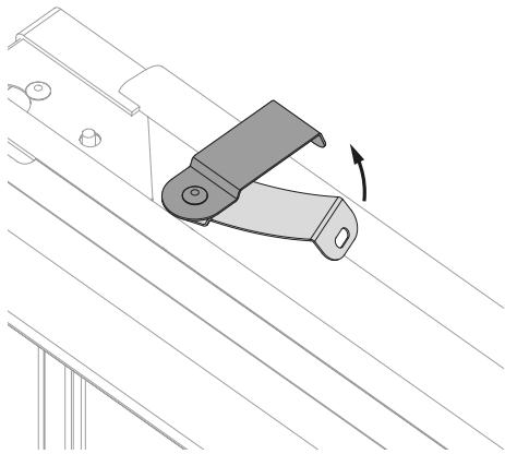
1. Rotate the four fastening plates on the damper 90° (to the upright position).
