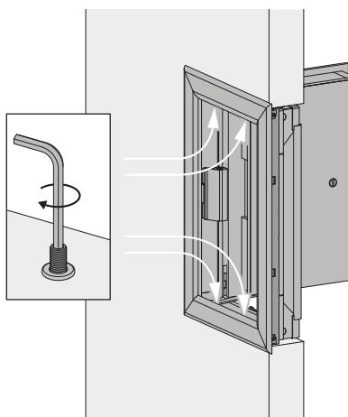
6. Tighten the position screws until just against the shaft, without distorting the frame. These screws prevent the Kamouflage AP from sagging in the opening.
