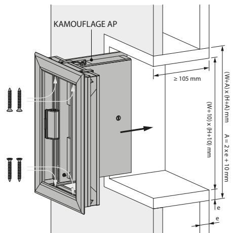
3. Example of mounting in a branch of a vertical duct, with a pre-wall finish.
