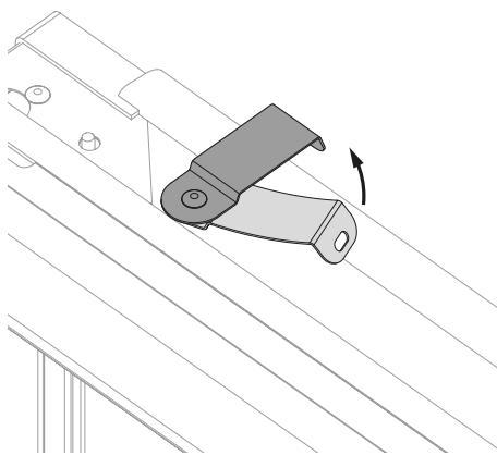
4. Rotate the four fastening plates on the damper 90° (to the upright position).
