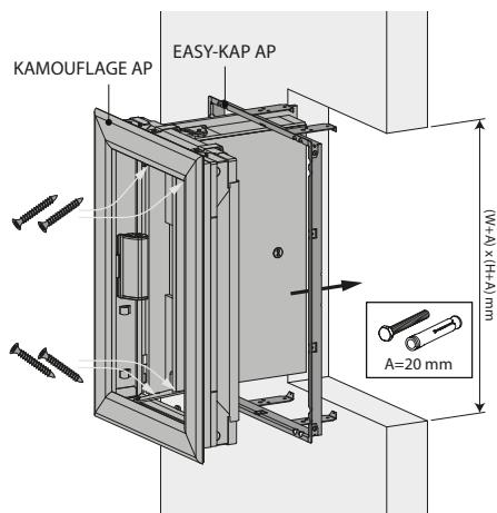
1. Make an opening with dimensions  $(W+20) \times (H+20)$  mm. Mortaring the mounting frame is not permitted.
