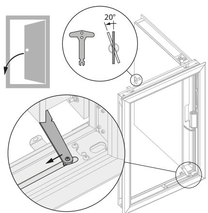
1. Turn the key 20° anti-clockwise. Push the actuating arm in the direction of the arrow and pull the shutter into its closed position.
